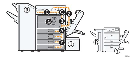
1. Press the key of the section from where you want to remove the jammed paper.
